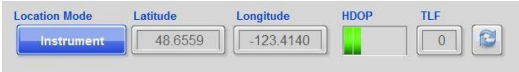
*Time To Last Fix (TLF)* is the number of seconds since the last valid GPS position. This number is usually 0 or 1. Higher numbers indicate poor signal quality. *Fix Quality* relates to the accuracy of the position reading. When this bar indicator is solid, the best possible accuracy has been achieved.
