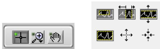
There are also icons in the lower right that control viewing options. Drag the plot view with the hand symbol. Set the size and location of the viewing area with the view selector.
