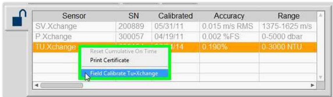
Invoke the turbidity field calibration dialog by right-clicking on the sensor table and selecting *Field Calibrate TU.Xchange*. This will take you to the field calibration dialog.
