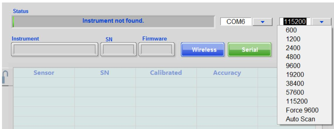
The *Port* field selects the serial port to which the instrument is connected. If uncertain about the port, check the ports in the Windows *Device Manager* or *Hardware Manager* found in the Control Panel. The *Refresh* selection at the end of the list forces a new detection of available ports. This is useful if a USB connection is made after SeaCast is launched.
