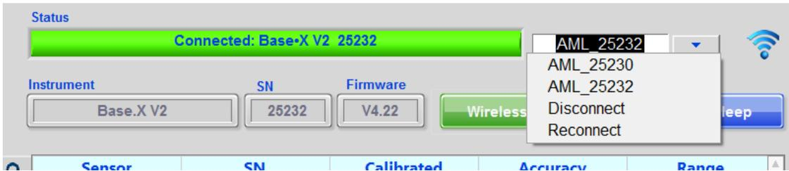
SeaCast establishes an ad hoc wireless profile to communicate with Data•Xchange. Any powered-up Data•Xchange modules in range will show up in the SSID control list; select the desired module from the dropdown. If the desired SSID does not appear in the list as expected, try refreshing the selection. Connection status will show progress, and signal strength will be indicated icon on the far right.
