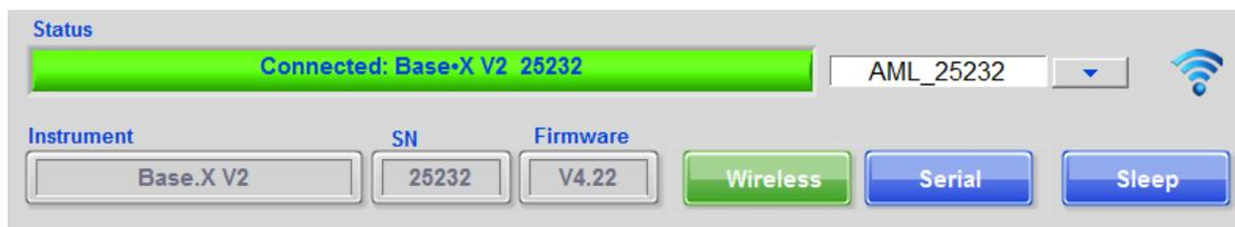
Communication indicators and controls set and monitor the two supported communication modes. Use the communication buttons to switch between them.
