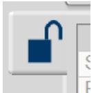
Once an instrument is connected and this icon is switched to the locked position, the connection time is greatly reduced. Use this feature if repeated connection cycles are anticipated with the same instrument and settings.
