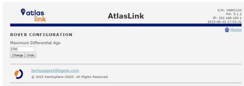
The “Maximum Differential Age” option controls the number of seconds after which the receiver will stop using a differential source once corrections are no longer being received.
