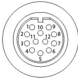
**Figure 2-2: Pin out assignments**
