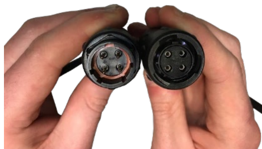
Female connector of the power supply unit and male connector of the breakout assembly
