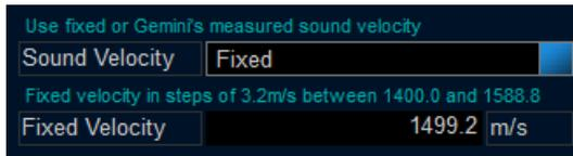
The above example shows the fixed sound velocity selected with a value of  $1499.2\text{m}\cdot\text{s}^{-1}$ . The software will round the value entered to a predetermined increment ( $3.2\text{m}\cdot\text{s}^{-1}$  or  $10.5\text{ft}\cdot\text{s}^{-1}$ ) which will be displayed on the Sound Velocity display on the User screen.
