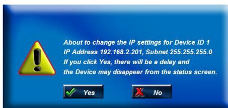
Clicking the `Yes` button will program the new IP address details into the Gemini. The new IP address followed by a reboot command will be sent. When the device reboots it will be using the new IP address, and therefore will not show up on the status display. Once the IP address of the computer has been changed back to its original settings the Gemini should once again appear on the status display.
