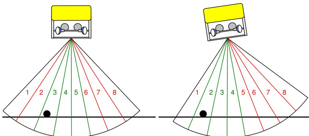
The above images illustrate an example using 8 profiler beams covering the full 130° swathe. The first image the reduced aperture swathe is defined by the Start and End Angles and is represented by the green beams (3, 4, and 5). Without Roll Compensation enabled the profiling will be done using beams 3, 4, and 5, regardless of roll. The consequence can be seen in the second image as beams 3, 4, and 5 do not cover the target pipe.
