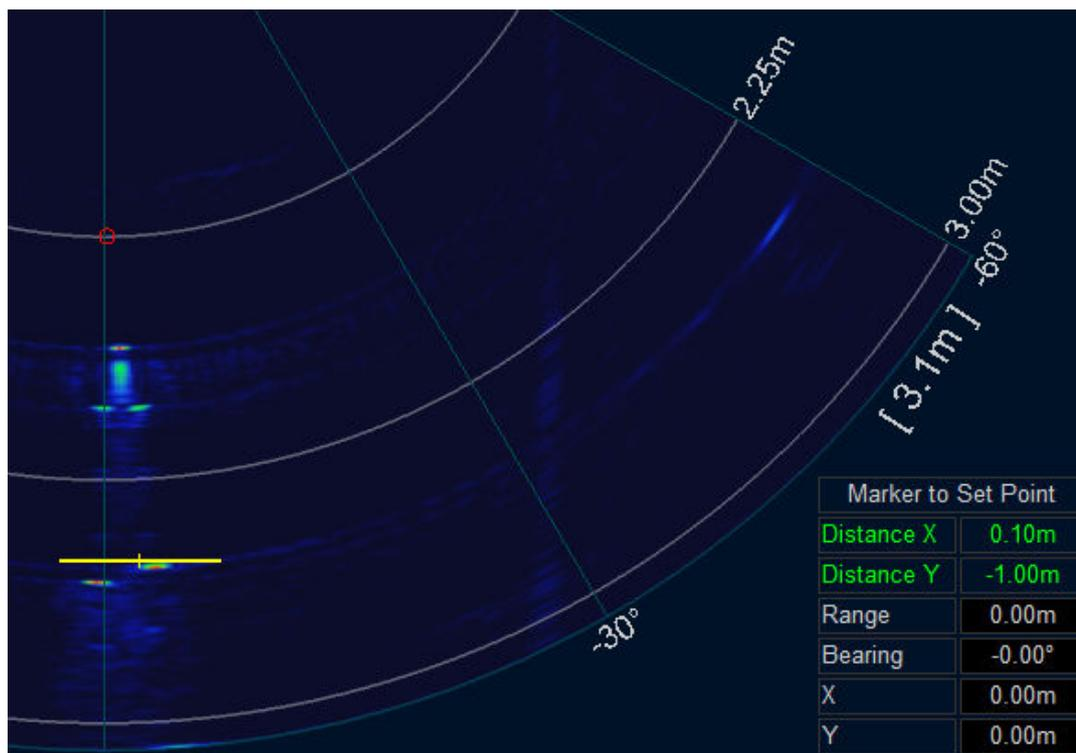
The Distance Marker range/ Y coordinate may be updated from an external sensor. Enabling the Distance Range from Sensor button will update the value whenever a configured sensor message is received. See Appendix D, *Gemini Software String Decode* for the appropriate Marker Range decode options.
