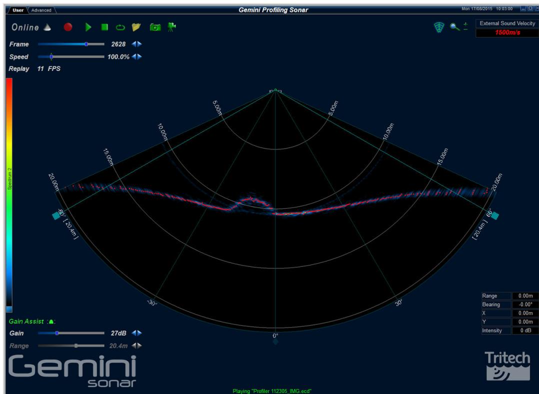
The cone in the middle of the display will show the profiler image that the Gemini Profiler is producing and the digitised points from the strongest returns. Around this display are the most commonly used controls. The CRP is shown as a small red circle.
