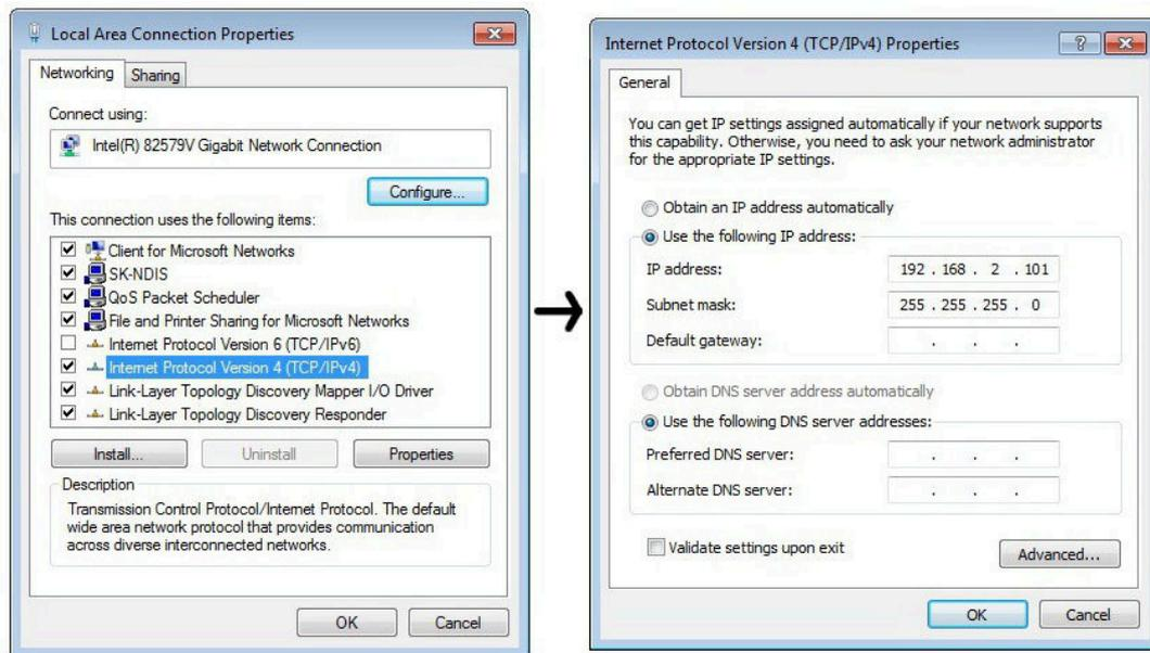
In the properties dialog which opens there will either be Obtain an IP address automatically OR Use the following IP address selected. If an IP address is already present, make a note of it before changing any values since it will be needed if the computer is ever restored to the previous network. Refer to appropriate section of this manual for the correct IP addresses to use.
