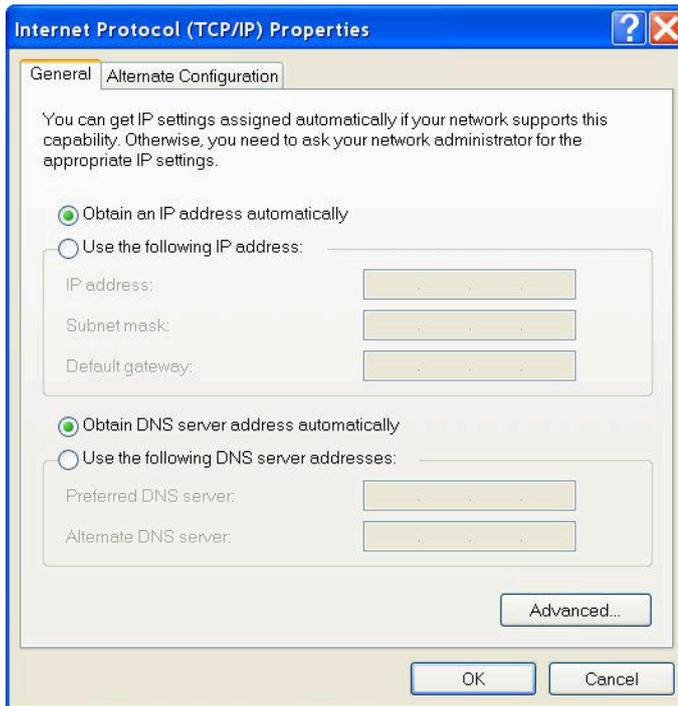
Make a note of the settings as currently used by the computer; these will be needed to restore the computer to any existing network. Refer to the appropriate section of this manual for the correct IP address to use.
