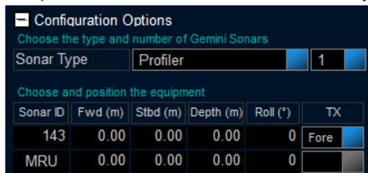
The configuration options allow for the selection and configuration of the profiling heads. Each head that is part of the system can be configured and the first step is to select the `Sonar ID` of the head to be altered. Each head can then be positioned in relation to where it is within the system (i.e. offsets can be input to compensate for the profiling heads being positioned either side of a ROV) by choosing the fore/aft (`Fwd (m)`) and port/starboard (`Stbd (m)`) offsets.
