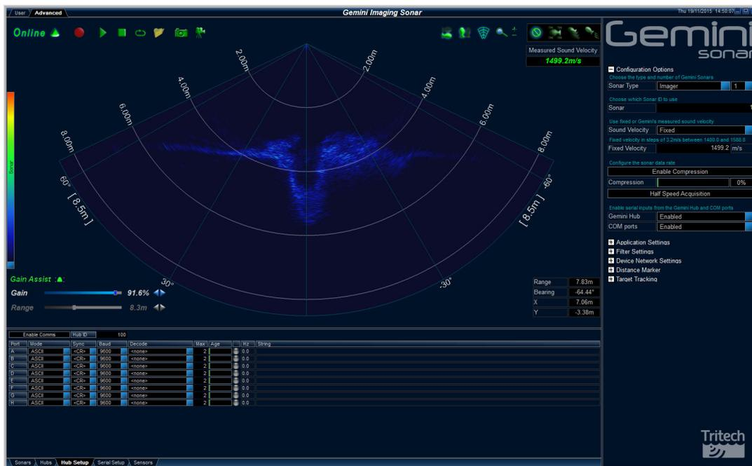
The Advanced screen shows more details about the Gemini system and allows certain options in the software to be configured. The screen is split into three areas: the User area; the System Data tabs, located at the bottom left hand side of the screen; and the Advanced Settings panel, which contains the majority of the configurable settings for the software.
