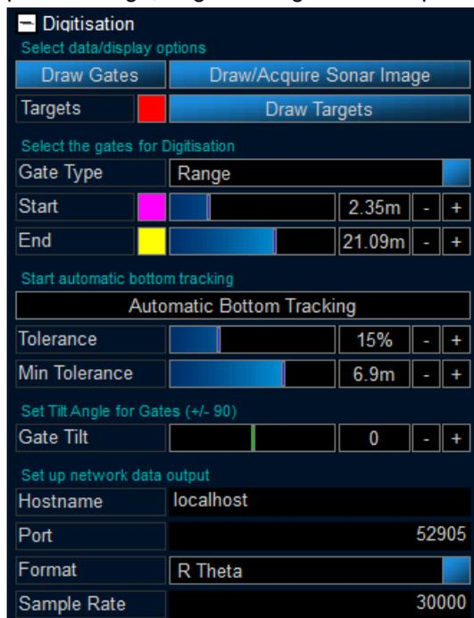
The `Draw Gates` button is used to enable/disable the drawing of the Start and End gates. This function does not affect the use of the gates which are still used for target detection when drawing is disabled.
