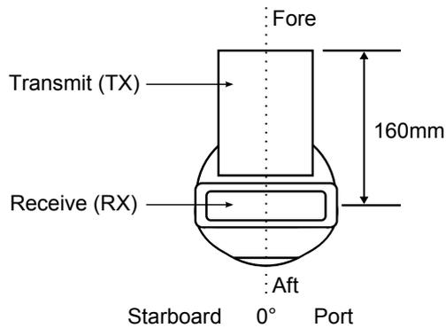
The view shows the profiler head as it would look from underneath the ROV with the front of the ROV at the top of the page, i.e., the profiler transmitter to the fore with the port side correctly aligned on the left.
