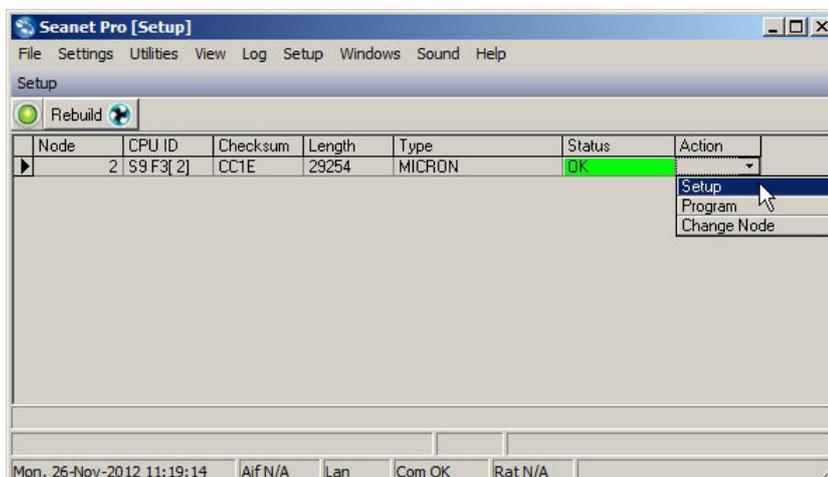
This will bring up the Digital Sonar Setup dialog. Locate the Comms Mode section in the lower right-hand corner and alter the Main or Aux ports of the Micron sonar as required.
