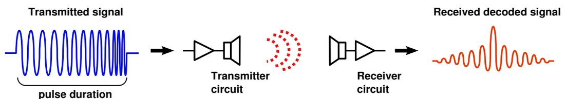
In a CHIRP system, the critical factor determining range resolution is the bandwidth of the CHIRP pulse which means the range resolution is given by:
