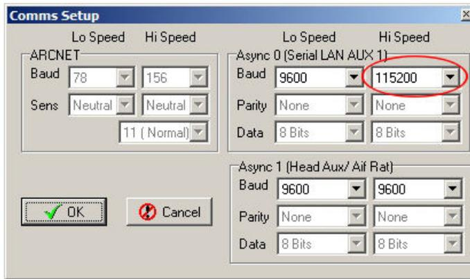
The Async 0 (Serial LAN AUX 1), Hi Speed is the only entry which should be changed.
