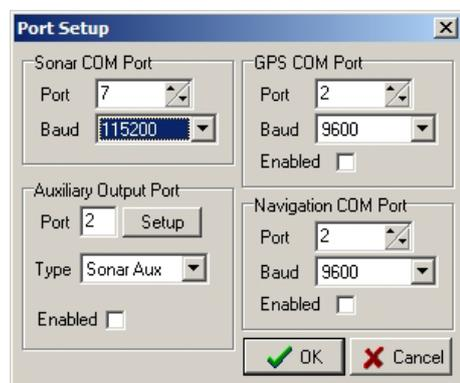
Under the `GPS COM Port` section select the computer serial port number and baud rate that correspond to the port which is receiving the GPS input. Once these have been set, ensure that `Enabled` has been ticked.
