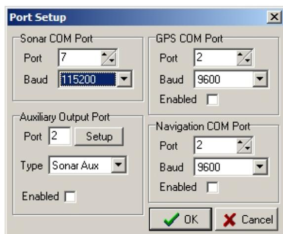
In the `Auxiliary Output Port` section, click on `Setup` to configure the COM port number and baud rate for the output altitude string. Once configured, tick the `Enabled` check box to open the port for the altitude data output. Ensure that the `Type` is set to `Sonar Aux` if outputting only Echosounder data (set to `Aux + Cursor` if cursor reporting is also required).
