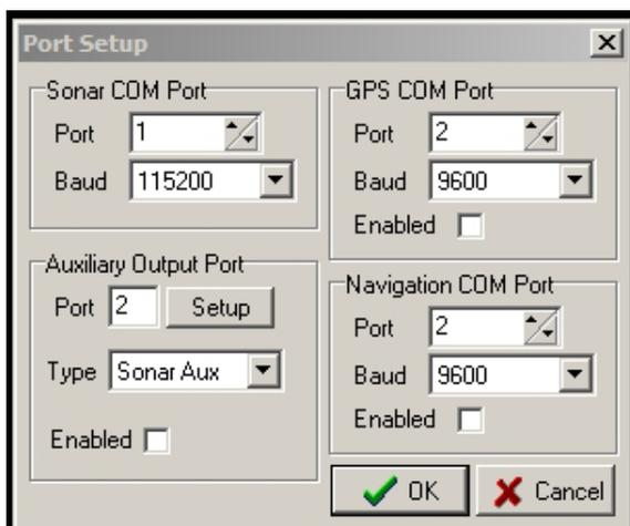
Select and configure the computer COM ports that the Micron, optional GPS and optional auxiliary device output (or cursor reporting output) will be connected to.
