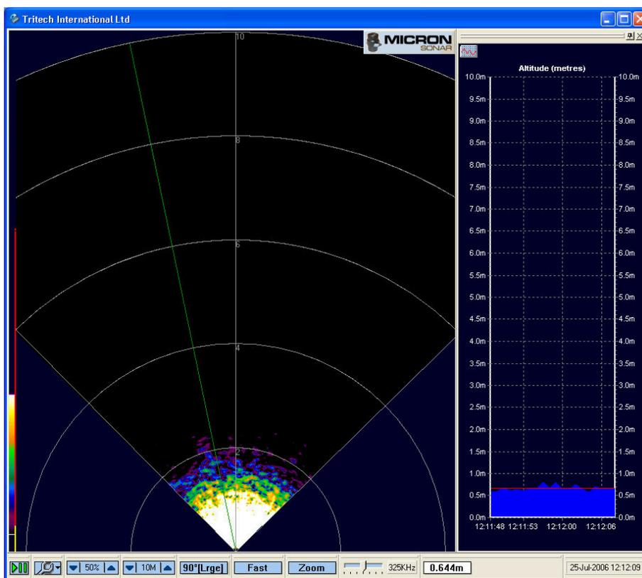
This chart can be docked on to the side of the window (as shown) or picked up and moved by clicking on the bar at the top of the chart and dragging it with the mouse. The chart display will auto-range depending on the value of the current altitude data. The maximum range for the Echosounder is 50m and the chart will change its range between values of 0-10m, 0-30m and 0-50m.
