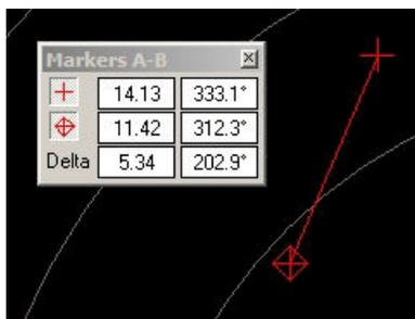
Adds a Markers A-B dialog to the screen where markers can be selected/de-selected and moved using the mouse. When a marker is first selected it appears on the origin of the sonar scan and if it is subsequently de-selected it will lose any of its positional data. When both markers are selected a line is drawn between them and the relative distance and bearing between them is shown.
