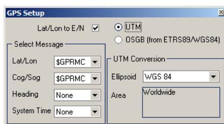
The GPS Setup dialog contains 5 drop-down menus for selecting NMEA 0183 message types for Latitude/Longitude, COG/SOG, Heading and setting System Time.
