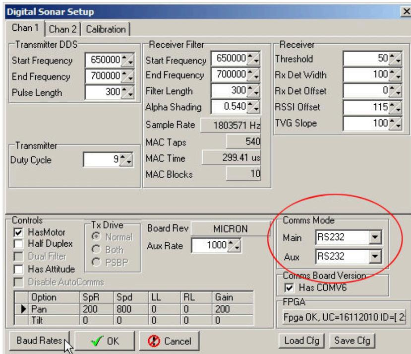
Once the new protocols have been selected, click on the OK button to apply the settings. If the Main port has been altered then the sonar will no longer be reachable and will have to be connected to the port or device that is using the new protocols.
