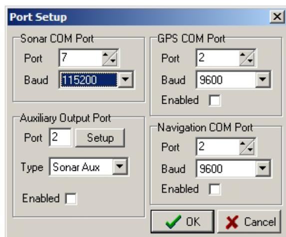
In the `Auxiliary Output Port` section, clicking on the `Setup` button will allow configuration of the COM port and baud rate. If outputting only cursor data, set the `Type` to `Cursor` otherwise set it to `Aux + Cursor`.
