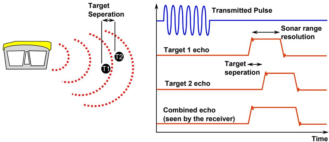
Using the example above, if two targets are less than 37.5mm apart then they cannot be distinguished from each other. The net effect is that the system displays a single large target, rather than multiple smaller targets.
