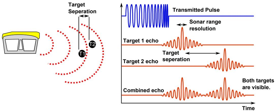
The response from the pattern-matching algorithms in the sonar means that the length of the acoustic pulse no longer affects the amplitude of the echo on the sonar display. Longer transmissions (and operating ranges) can be achieved without a loss in range resolution.
