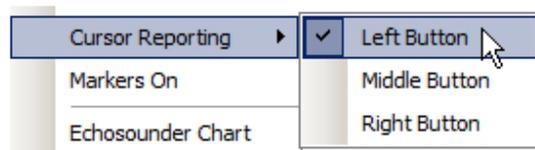
By clicking on the sonar display window with the selected mouse button the range and bearing position of the mouse pointer is sent to the remote computer via the allocated COM port. To report on the position of a particular target on the sonar display, hover the mouse pointer over the target and click with the mouse button to activate an output string.
