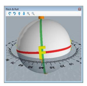
The forward, aft, port and starboard of the vessel are indicated on the model with F,A,P & S respectively. The arrow shows the current vessel heading overlaid on the compass.
