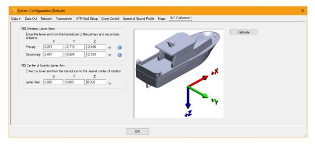
On this tab the lever arm offsets are entered for the INS, these are used by the inertial engine to calibrate and align the system.
