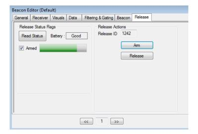
This will set a 60s window where the beacon must then be released. When the release command is sent a prompt will ask to confirm the release.
