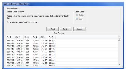
In the data preview window, select the column that contains the depth value by clicking on the relevant column header. The depth units will default to meters, if the data is in decibars then ensure the Depth Units is set accordingly. Once selected, press 'Next' to continue.
