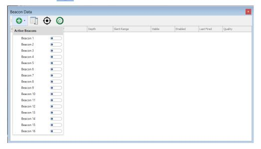
This is the primary control and monitoring window for the system, the beacon configuration is set within Beacon Editor.
