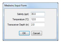
Enter the parameters. The result is automatically placed in the VOS text box.
