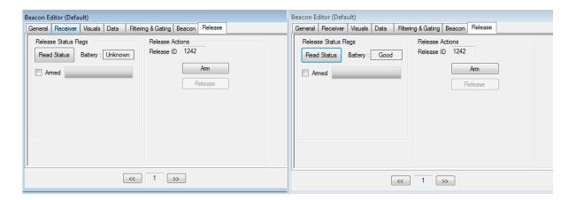
When the Arm command is pressed providing the ID is correct and a valid reply is received the release button will become active, the ARMED flag will be set and a countdown bar will start travelling across.
