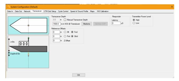
The following offsets are available: Forward/Aft (m), Port/Starboard (m), Z (Height m). Transducer depth (m) below water line.
