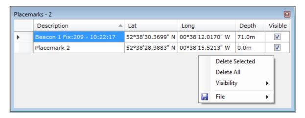
Place marks are designed to offer the operator the ability to mark and record places of interest or events typically in Eastings and Northings (for reference) with the depth of the reading appended. The above example is shown with the context menu displayed (right mouse click).
