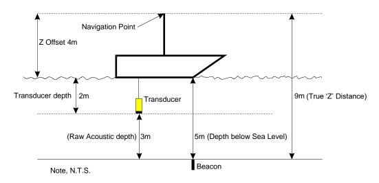
The Navigation Point is the point on the vessel where all navigation measurements are referenced to; in above example, the top of the mast.
