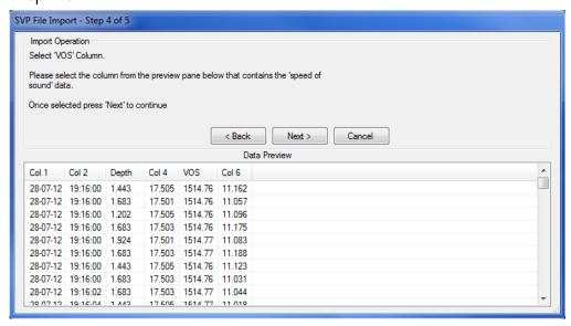
In the data preview window, select the column that contains the velocity of sound value by clicking on the relevant column header. Once selected, press 'Next' to continue.
