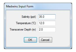
Enter the parameters for the calculation and click 'OK' to perform. The result is automatically placed in the VOS variable.
