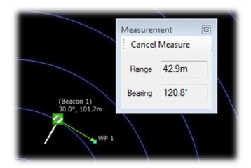
The Measurement Tool can be used to measure between any two points on the plot screen, a range and bearing will be displayed in the measurement window.
