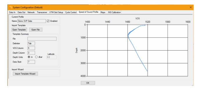
Once a Sound Velocity Profile has been loaded and enabled, the system will automatically calculate the optimum velocity of sound value for each beacon, based on the current depth of the beacon. This value will be continually updated as the beacon depth changes.
