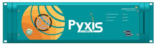
Easytrak Pyxis is an advanced inertial Ultra Short Baseline (USBL) positioning and tracking system which incorporates Sigma Spread Spectrum Technology to provide a secure acoustic link The console integrates the main PC and INS processing unit and provides control and interfaces for the system. The console also provides power and communications to the Easytrak Pyxis Transceiver and GNSS antennas.
