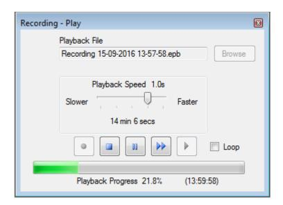
The record and playback function allows the operator to record the tracking and all peripheral interfaces in real time. To have the facility to play back the logged data for review. As the data is recorded in raw format the data sets can be re-created with new offsets, smoothing levels, etc. to produce a different final data set.
