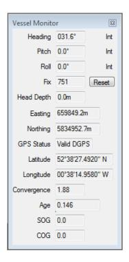
The Vessel Monitor also indicates if internal (Int.) or external (Ext.) heading, pitch and roll are selected.
