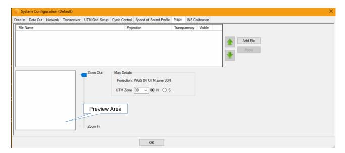
Multiple overlay files may be added. Each file can be moved up or down the overlay order and can be set to the required transparency to enable optimal viewing.
