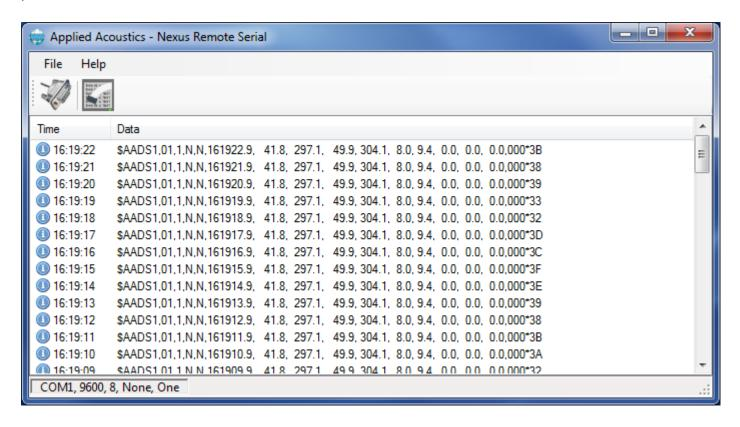
The application may be configured to output on any available serial port and at any required baud rate and data format.
