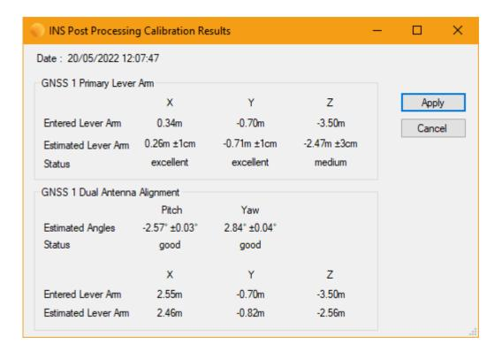
Following applying the new lever arms the Pyxis system will require re-boot and INS alignment.
