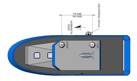
TRANSCEIVER ALIGNMENT FACING BOW. GNSS CAN BE INSTALLED PORT / STARBOARD WITH CORRECT LEVER ARM OFFSET.
