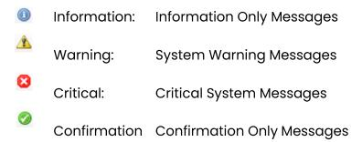
The Event Log can be filtered to display only the desired level messages. By selecting one or more of the message type icons in the tool bar to view messages. Filters can be removed to display all messages.
