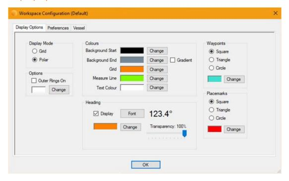
The Display Options tab allows the operator to configure the display to their preference for the local environment. For example - by altering the colour scheme 'workspaces' can be created for day and night operations.
