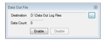
The output message generated by nexus, and sent out via the data out port, may be logged to a text file.
