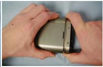
With the camera on a flat surface, hold the body housing in one hand and the head housing in the other then simply pull apart.
