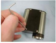
Turn the camera underside up and remove the 4 x 2.5mm hex bolts from the base-plate.
