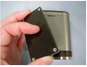
The base-plate can now be removed revealing the ends of the nylon securing cord.
