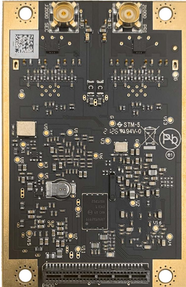
**Figure 1-3: Vega 60 GNSS OEM Board**
