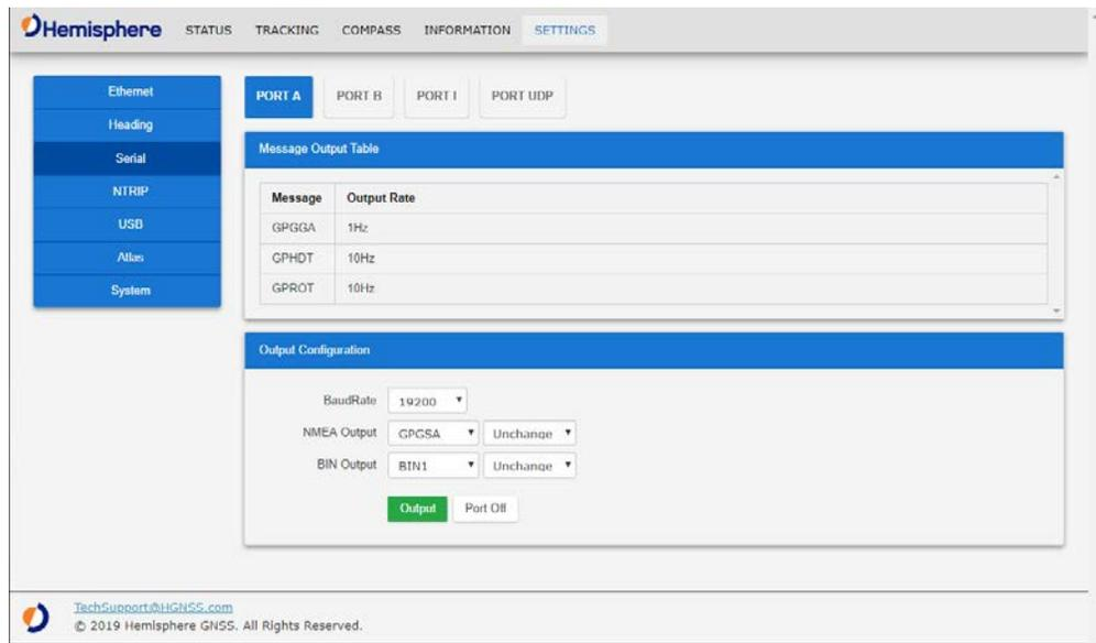
The screenshot shows the Hemisphere web interface with the 'SETTINGS' tab selected. On the left, a navigation menu includes Ethernet, Heading, Serial (highlighted), NTRIP, USB, Allan, and Syslog. The main content area is for 'PORT A' configuration. It features a 'Message Output Table' with the following data:
