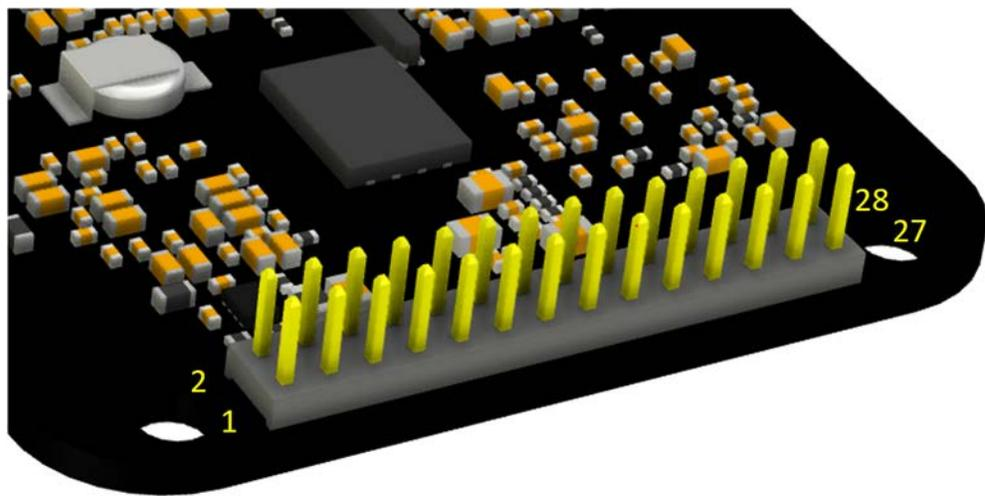
**Figure 2-5: Vega 28 pin layout**
