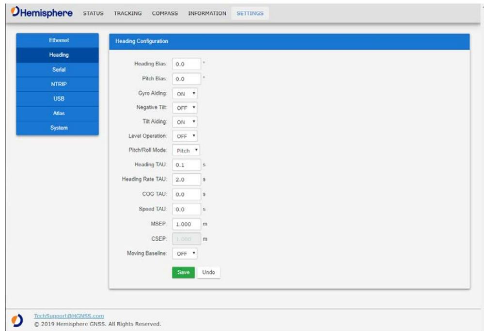
The screenshot shows the Hemisphere web interface with the 'SETTINGS' tab selected. On the left is a navigation menu with options: Ethernet, Heading, Serial, NTRIP, USB, Atlas, and System. The main content area is titled 'Heading Configuration' and contains the following settings:
