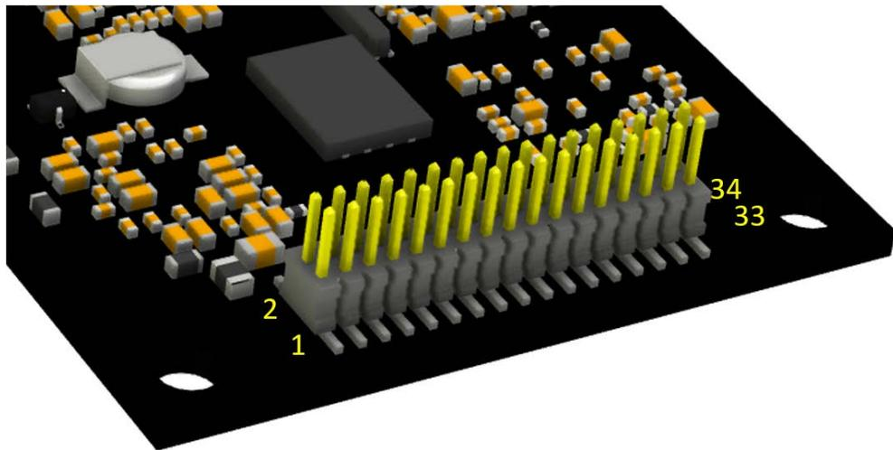
**Figure 2-6: Vega 34 - 34-pin header layout**
