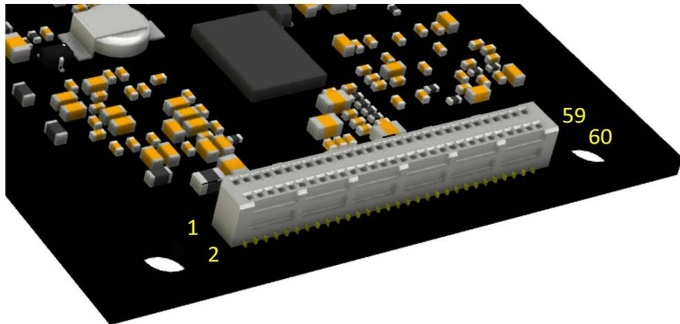
Figure 2-7: Vega 60 60-pin layout
