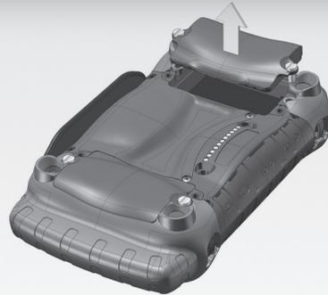
**2** Loosen quarter turn latches to open battery compartment door.
