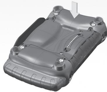
**4** Close battery compartment. Replace door, tighten latches.
