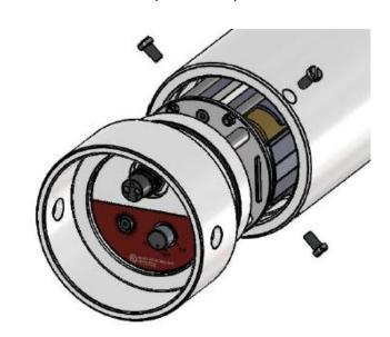
(3) Remove battery retaining bars.
