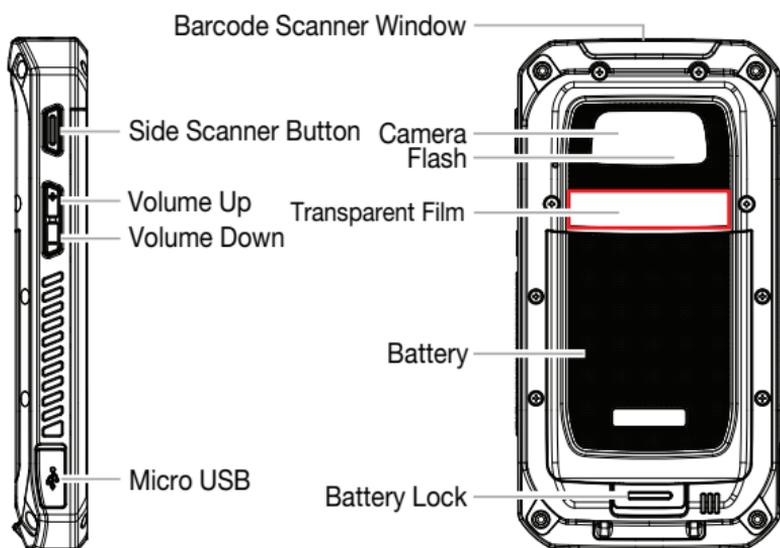
**NOTE** Do not remove transparent film unless you are using the pistol grip accessory
