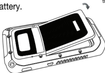
The battery is secured by a red slider. Move the slider to the right to unlock the battery.
