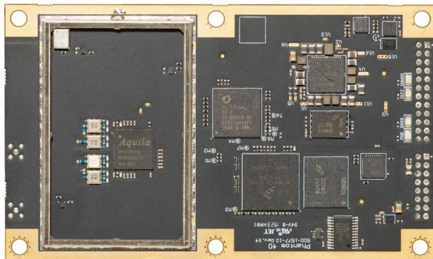
**Figure 1-2: Phantom 40 GNSS OEM Board**
