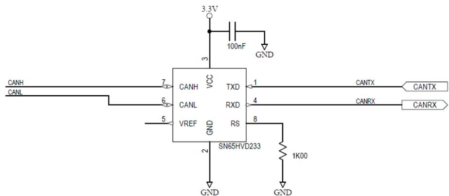
**Figure 2-5: Phantom 40 CAN design example**
