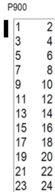
**Figure 2-3: Phantom 40 24-pin header layout**
