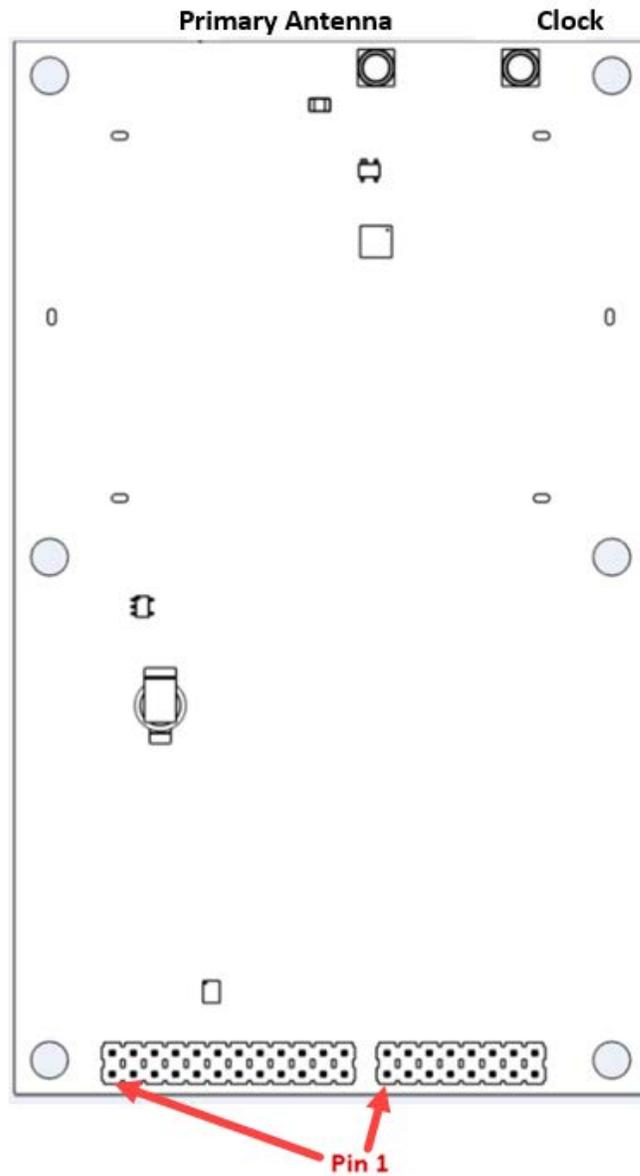
Figure 2-2: Phantom 40 Connectors
