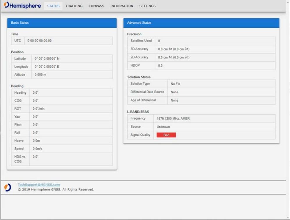
The screenshot displays the Hemisphere Phantom 40 WebUI Status window. At the top, there are navigation tabs: STATUS (selected), TRACKING, COMPASS, INFORMATION, and SETTINGS. The main content area is divided into two panels: Basic Status and Advanced Status.
