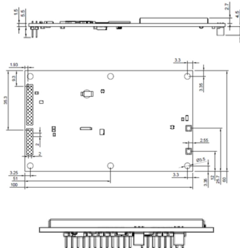
**Figure 2-1: Phantom 40 mechanical layout**
