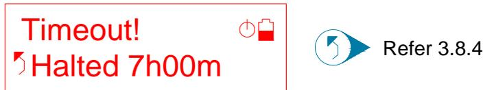
The Smart Switch terminated beacon charging. The Smart Switch monitors overall beacon charging time. If the overall charging time exceeds a defined time limit or “timeout”, the Smart Switch terminates beacon charging. This ultimate safety feature is independent of the beacon chargers own timeout.
