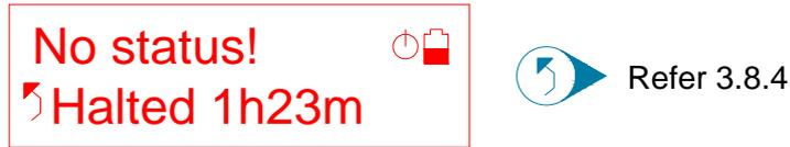
The Smart Switch does not detect fast charge status information from a connected beacon. Check the following: -
