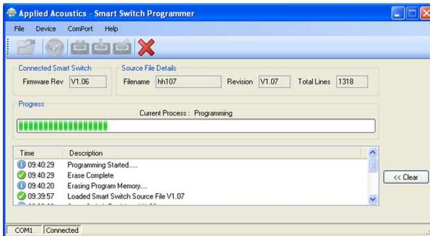
8. When programming is complete reset the Smart Switch.
