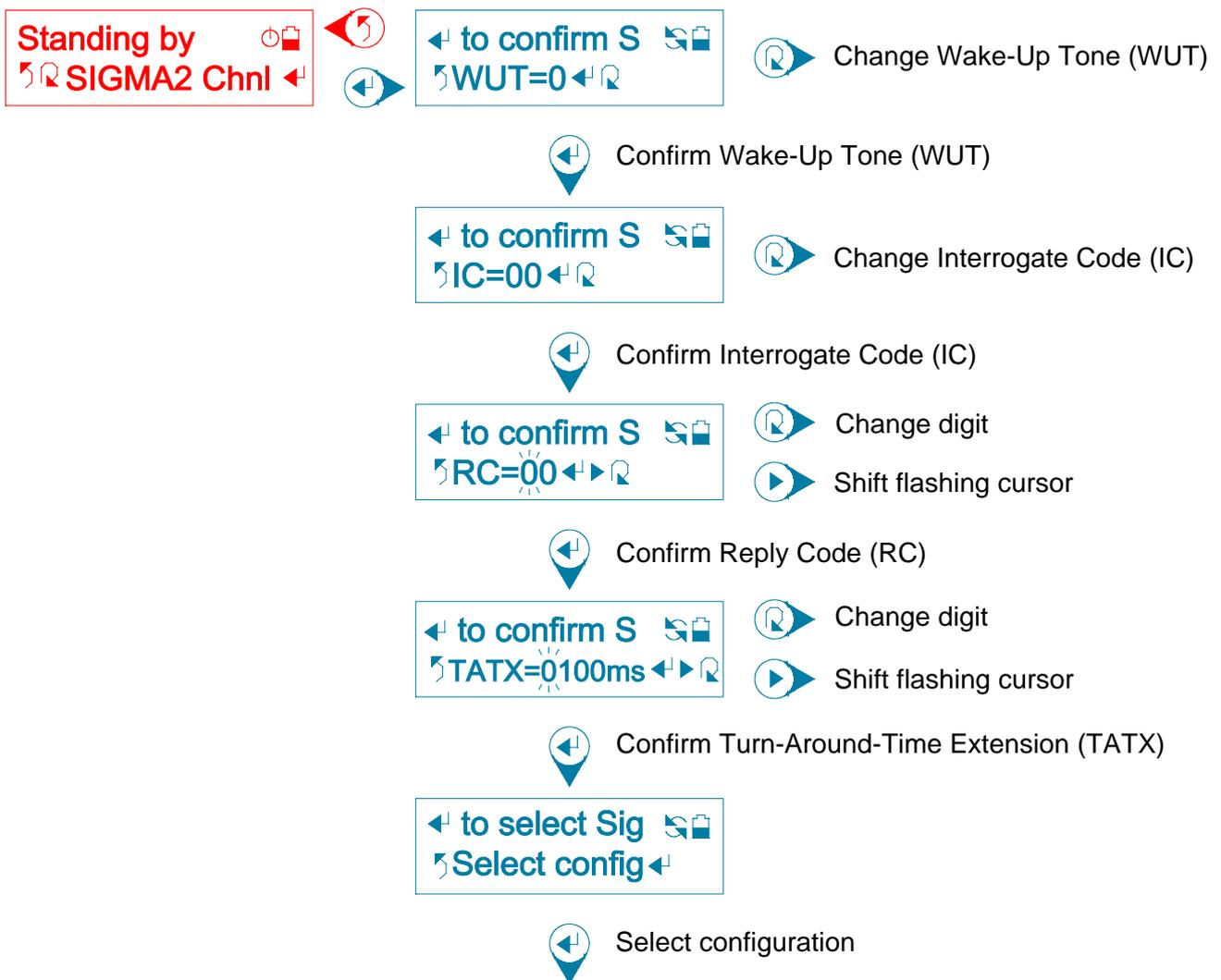
First, a user selection for Wake-Up Tone (WUT) is displayed. Press **←** to return to the previous tier sub menu option “SIGMA2 Chnl”. Press **→** to change the Wake-Up Tone (WUT) 0 through 7. Press **↓** to confirm the Wake-Up Tone (WUT). The Smart Switch will display a “Confirmed!” message.
