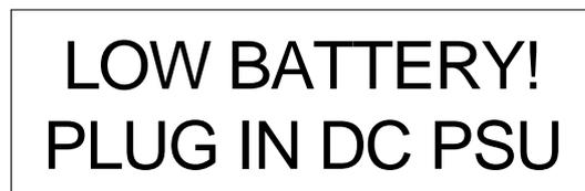
The Smart Switch will be non-operable until the internal battery has been partially charged. Insert the included 30VDC power supply unit. After a period of trickle charging, the Smart Switch will reset and become operable.
