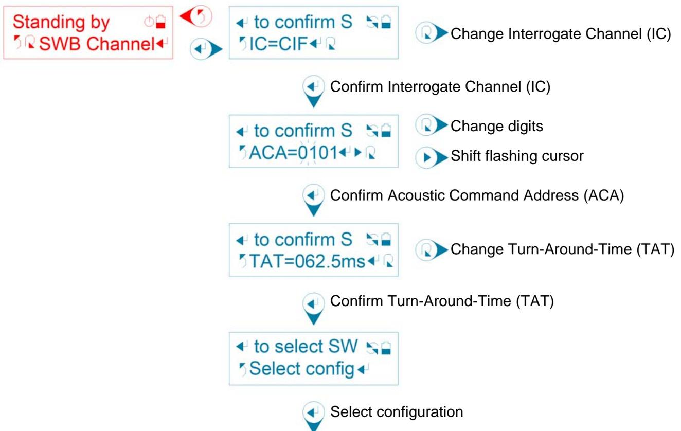
First, a user selection for Interrogate Channel (IC) is displayed. Press **⏪** to return to the previous tier sub menu option "SWB Channel". Press **⏩** to change the Interrogate Channel (IC) CIF through MF14. Press **⏩** to confirm the Interrogate Channel (IC). The Smart Switch will display a "Confirmed!" message.
