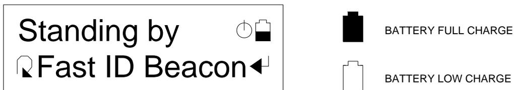
Operational life is typically 2 days with constant use and with the backlight enabled. Standby life is typically 5 months.
