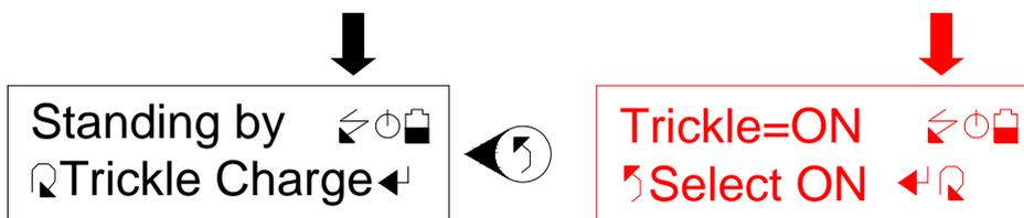
The Smart Switch continually monitors the 30VDC power supply unit while trickle charge is active. If the Smart Switch does not detect the 30VDC power supply unit, the electronic switch within the Smart Switch will open and the L.C.D. charge active icon will be removed. Trickle charge will have to be re-activated if required.
