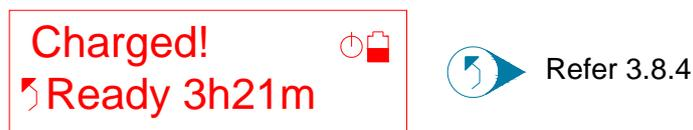
Beacon onboard fast charger indicates battery is fully charged, together with overall charge time in hours and minutes.
