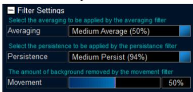
The `Averaging` filter applies an average over a number of images received from the sonar. It has the effect of removing random noise and rapidly moving targets from the image.
