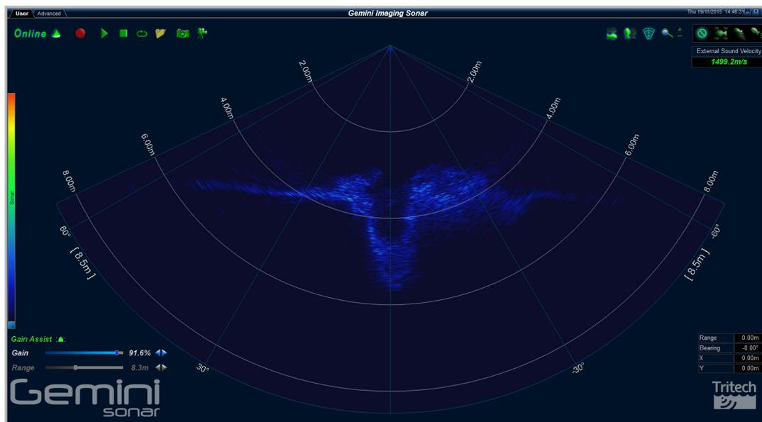
The 130° cone in the middle of the display shows the sonar image that the Gemini Sonar is producing. Around this display are the most commonly used controls.
