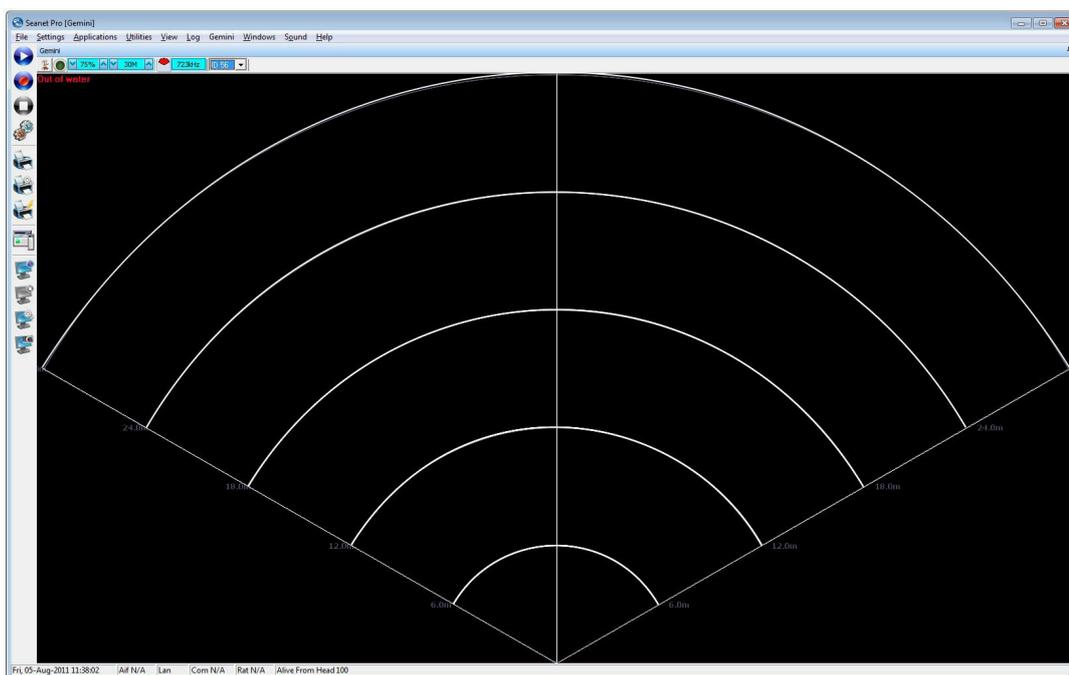
The Gemini Sonar display is very similar to the standard Sonar display used for *Tritech International Ltd* mechanical sonar heads such as *SeaKing* and *SeaPrince*. However, the Gemini Sonar has a fixed scan sector of 130° and unlike the mechanical heads does not have option for scan sector size and position adjustments. Therefore these function controls have been omitted from the settings bar.
