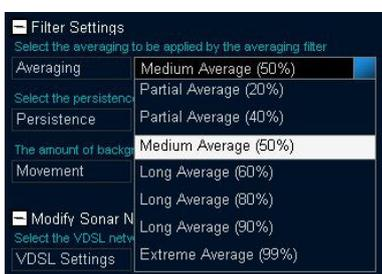
The `Persistence` filter retains decreasing amounts of earlier images as well as the current image. It has the effect of highlighting movement in the images, which appears as a decaying “snail trail” behind the moving object.
