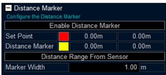
Enable the feature by clicking the `Enable Distance Marker` button. This will draw the `Distance Marker` as a horizontal line and the `Set Point` as a small circle in the Gemini data view.
