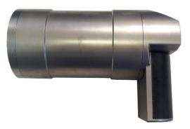
Operating at 620kHz the Gemini NBI is able to produce images with 10mm range resolution while the 0.5° horizontal angular resolution results in an extremely sharp sonar image. Where monitoring your position relative to a known target is the objective, and not general obstacle avoidance, then the Gemini NBI can help guide you safely to the desired target.
