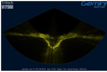
Tritech's Gemini NBI Image of an excavation operation showing the clear visibility of a cable being trenched (image courtesy of Reef Subsea Dredging & Excavation).
