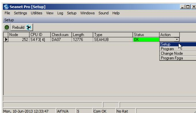
**Figure 4.18. SeaHub Action Menu in Node Table**
