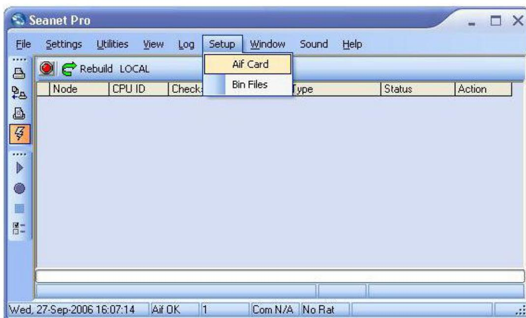
**Figure 4.6. Seanet Setup, Setup menu**
