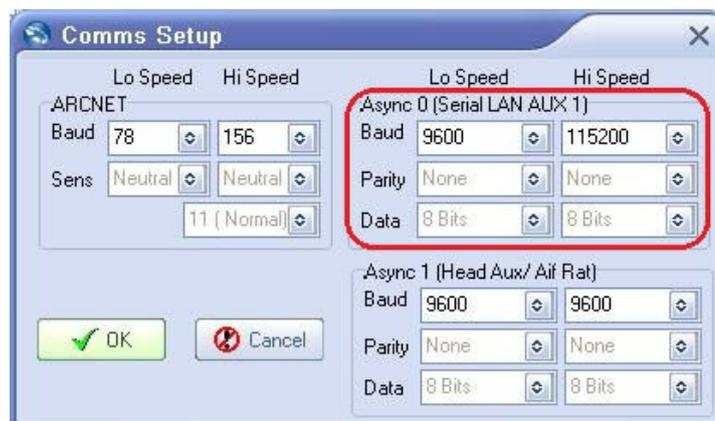
**Figure 4.11. AIF PCI Card Baud Rates, AUX 1**
