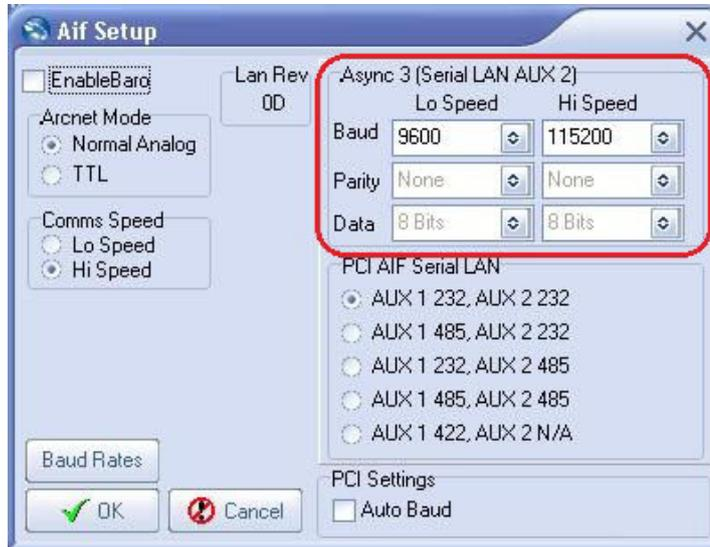
**Figure 4.12. AIF PCI Card Baud Rates, AUX 2**
