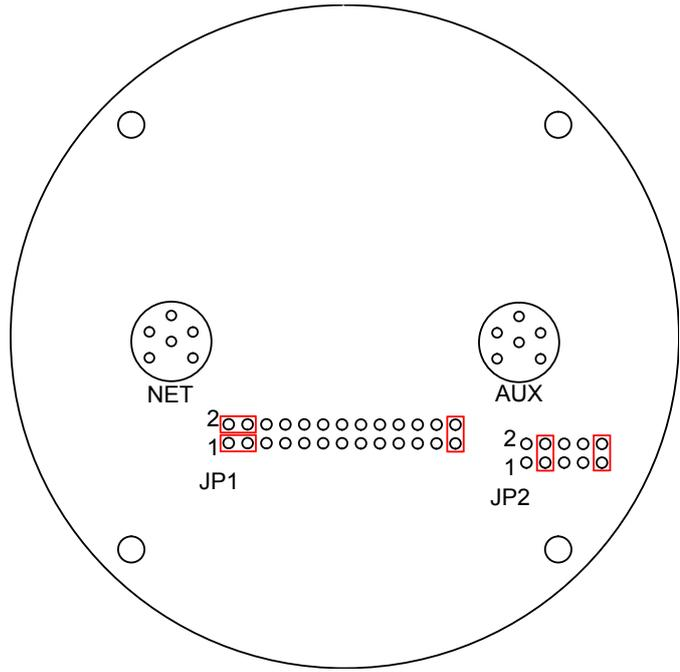
**B.2. RS232 Jumper Links for DFS, DST, ROV Sidescan & Sub-bottom Profiler**
