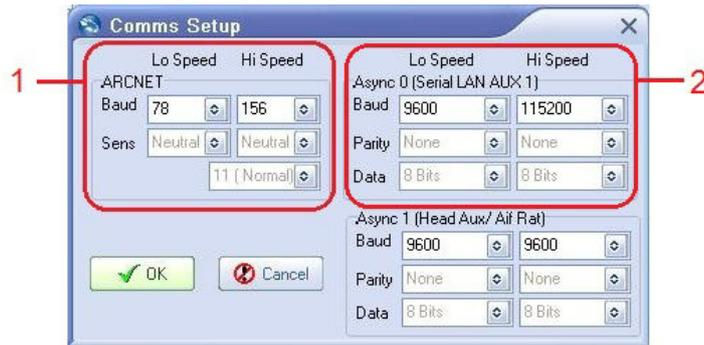
**Figure 3.2. Comms Setup Dialog for ARCNET & RS232**
