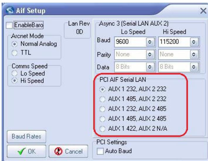
**Figure 4.9. AIF PCI Card Setup, Channel Selection**
