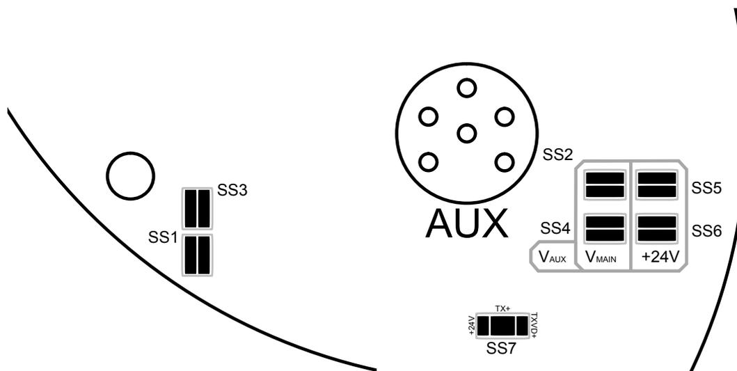
SS1 and SS3 are located in the lower left section of the PCB.
