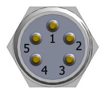
PIN 1. External Trigger Input / RS232 RXD
