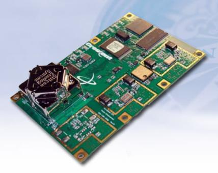
Create a more dynamic navigation solution through Hemisphere GPS' advancements in Crescent® Vector™II technology. The enhanced Crescent Vector II OEM board brings a series of new features to the patented receiver technology including heave, pitch and roll output, more accurate timing, lower phase noise and an improved accelerometer. Use the new Crescent Vector II OEM Board for all applications that require reliable heading and positioning.
