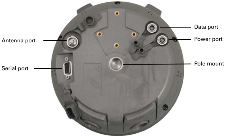
Figure 2: S320 ports and connectors
