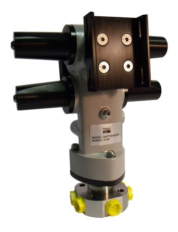
The Tritech PT3636-HD pan and tilt unit is designed with the hydraulic connections located on the mounting base, which allows the unit to be installed using rigid rather than flexible piping. By using rigid piping the system offers reduced interference and smooth operation of cameras or lights and increases the efficiency and reliability of the unit.
