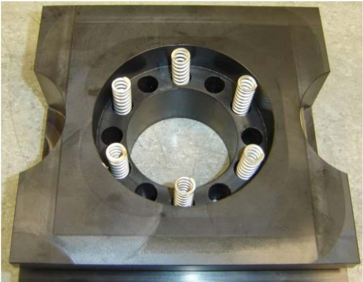
Figure 5.5. Springs in Place
