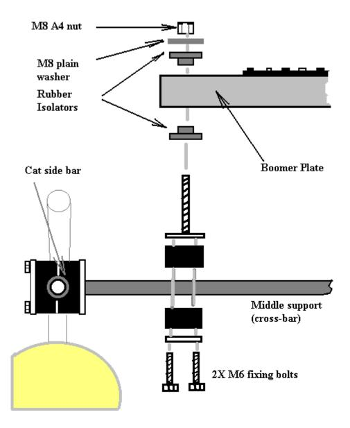
Fit the two rubber isolators on each side of the Boomer plate and secure with stainless A4 M8 nuts and flat washers.
