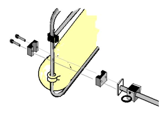
Bolt the front towing cross member to each catamaran floatation side using the plastic isolation clamp and 10mm bolts. Note bolt heads should face outwards from Catamaran sides. Proceed with rear cross member (refer to parts designation picture for completed unit view).
