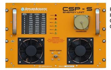
Relay Switchable HV Capacitor Banks HV Energy Switch O/P Monitoring O/P Connection
