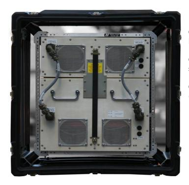
Connect **CONTROL** Link Cable (Left Hand Side) as shown.
