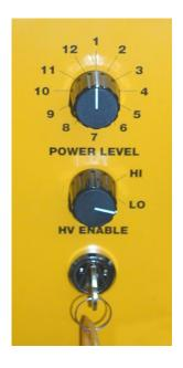
The maximum repetition rate is governed by the charge rate (1500 Joules per second) and the amount of capacitance selected. For example, at 300J / shot the CSP-D models will run at 5 PPS. At 1200J (or 1250J), the CSP-D 1200 and 2400 will operate at 1 pulse per second, with a little in reserve.
