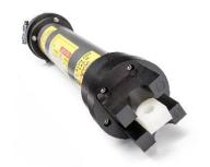
**The 500 Series** release beacon provides the means by which scientific, survey or operational equipment can be deployed or reliably retrieved from its anchored seabed mooring.
