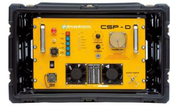
**The CSP-D** is a seismic energy source for boomer and sparker applications in three variants, the CSP-D700, CSP-D1200 and CSP-D2400. Each unit has the same chassis and 1500J/second HV engine.
