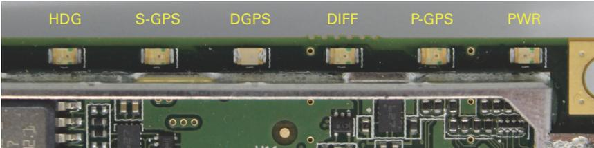
**Figure 2-3: Onboard LEDs**
