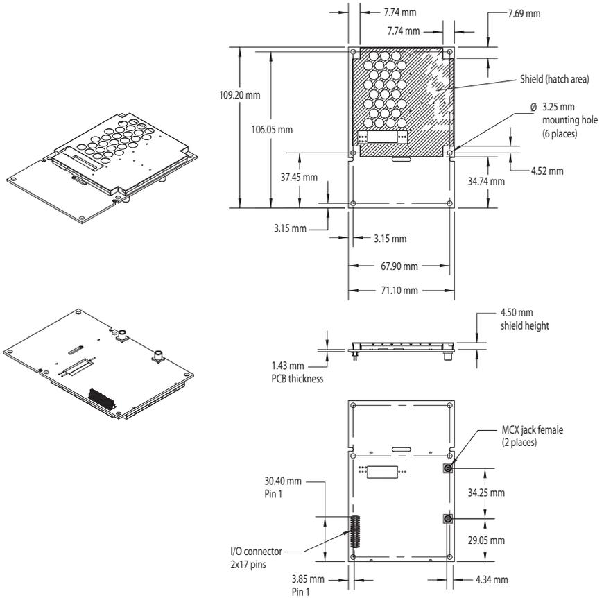
**Figure 2-1: H200 mechanical layout**
