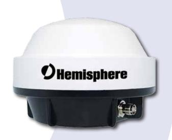
The A43 antenna adds precision, reliability, and value to our leading Eclipse™ GPS technology. The A43 antenna is a multi-GNSS precision antenna and is ideal for various applications including construction survey, RTK positioning and navigation, precise guidance, and machine control. Use the A43 antenna in challenging environments (such as near buildings and foliage) as it has superior multipath mitigation, stable phase center and strong SNR's even at low elevations.
