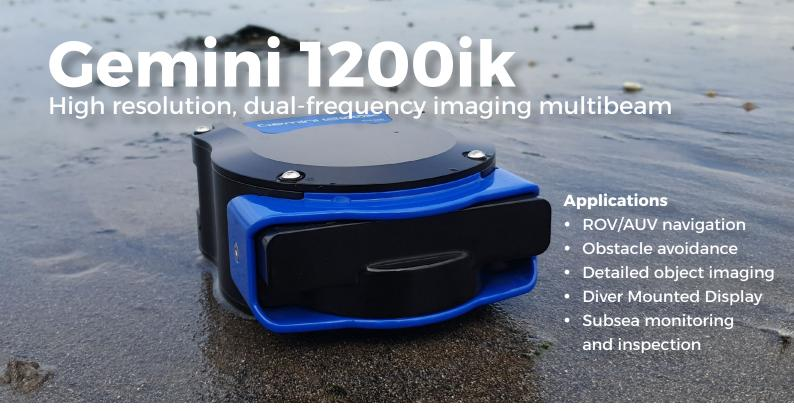
The Tritech Gemini 1200ik multibeam sonar operates at two acoustic frequencies, 720kHz for long range target detection, and 1200KHz for enhanced high resolution imaging at shorter ranges. Switching between acoustic frequencies is done either manually or automatically at a range set by the user.
