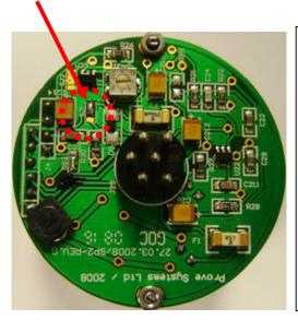
TO ENABLE VIDEO OUTPUT (Without Amplification) Link solder pads 1 & 2 together - Amplification & video filter are OFF DEFAULT SETTING
