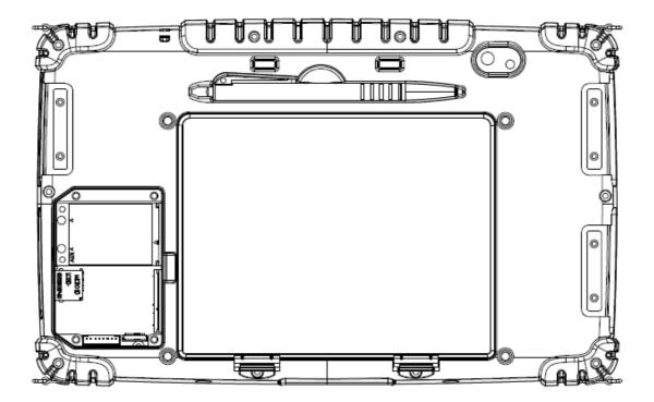
Install the antennas. The ALGIZ 10X has two WWAN antennas connected to the LTE card. Install the antennas according to the picture.
