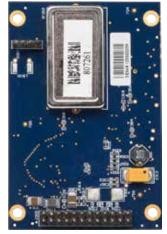
Provide a reliable source of differential corrections with the SBX-4 radiobeacon board that augments a separate GPS receiver with free accuracy-improving correction data from networks of beacon stations located throughout the world.
