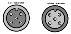
Figure 2-9: NMEA 2000 cable pin assignment
