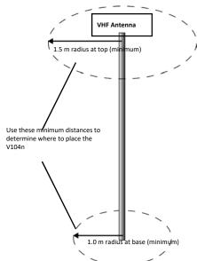
Figure 2-1: V104n distance from nearby VHF radios
