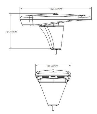
Figure 2-7: V104n Dimensions with Adapter
