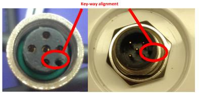
Rotate the cable ring clockwise until it is secured firmly to the unit (handtighten).
